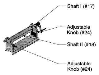
Figure 1 -- Adjusting the Material Gap
